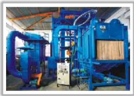
Airless 10 Rotor Type Blasting M/c for 'I' Section Cleaning
