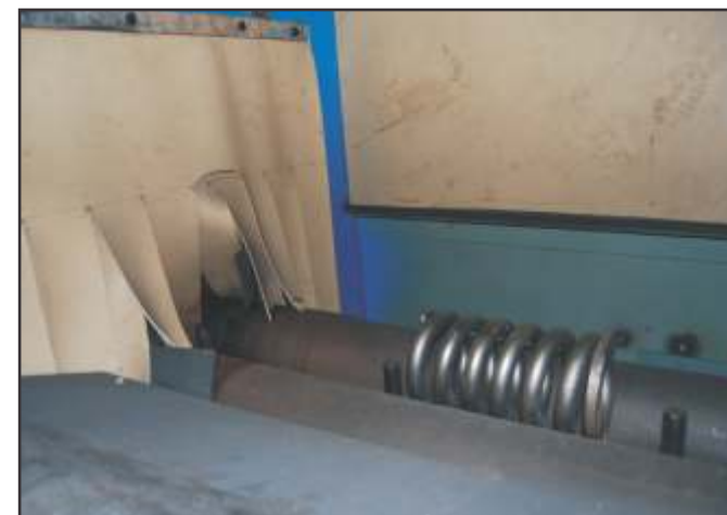
Coil Spring on Roller inside Machine
