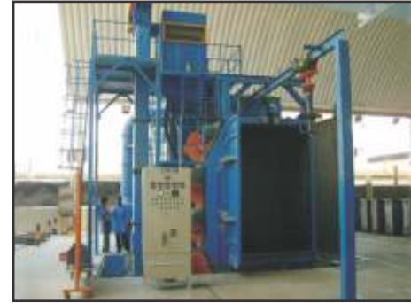
'T' Hanger Type Shot Blasting M/c with Motorized Hoist for Electric Transformers
