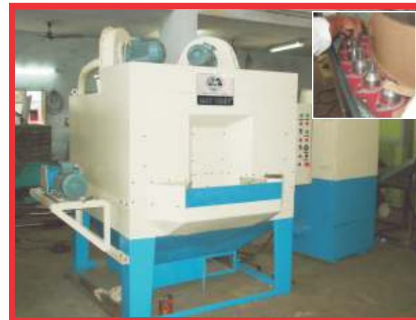
Airless 2W Cabinet Type Shot Blasting M/c with Nylon Shots for Servo Motor Starters
