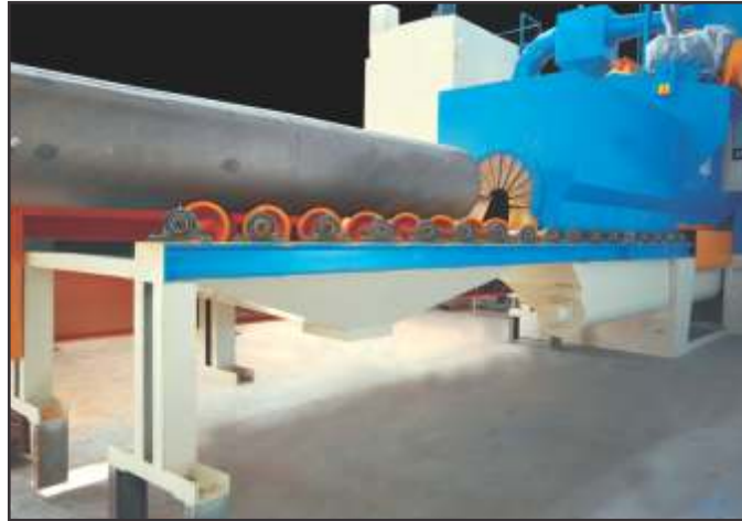
Airless 2 Wheel Diabola Type Shot Blasting M/c for Pipe Cleaning
