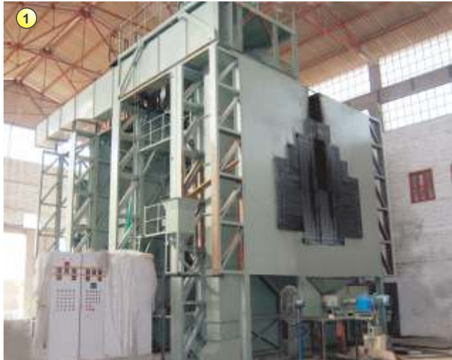
Airless 30 HP 10W Hanger Type Huge Special Shot Blasting M/c for "U" Shell Drum
