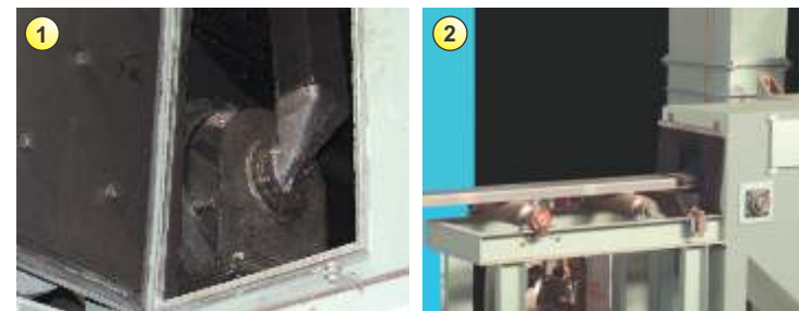
Airless 50 HP 6W Special Shot Blasting M/c with Airless Magna Valve for Shot Flow Control for 'C' Channels
